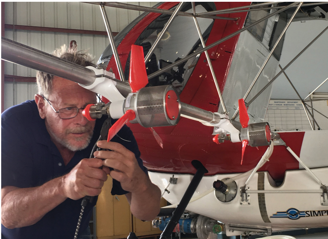
Director of Aviation Maintenance Jay Wilson adjusts the Simplex 8500 larviciding system after it was installed on an MD-500 helicopter. The dual-boom system was designed and crafted by the District's maintenance staff.
