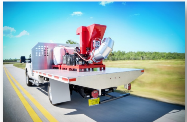
Rear view of the truck mounted Buffalo Turbine Mister/Sprayer
