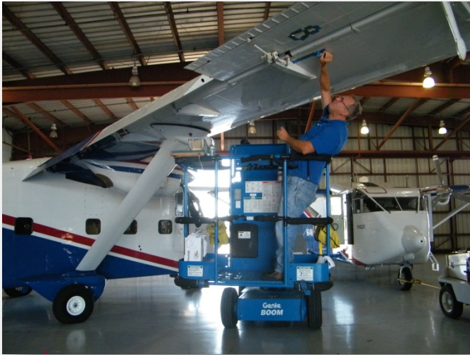
Aviation Assistant Jon Morris performing corrosion work on one of the District's Skyvans
