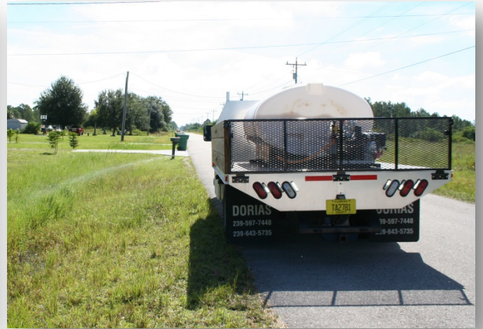
CMCD personnel larviciding a ditch via a truck outfitted with a 400 gallon larviciding unit
