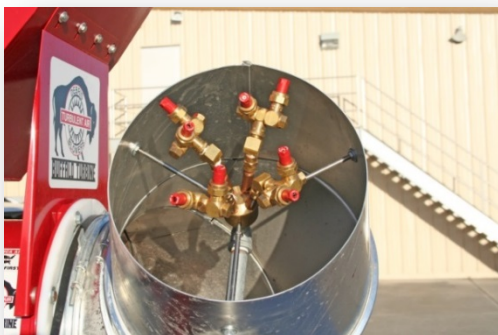
Hydraulic nozzles on the Buffalo Turbine Mister/Sprayer
